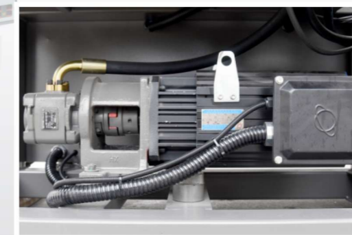
Servo motor and gear pump
