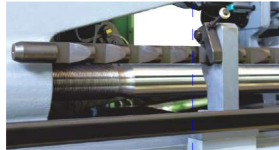
Auto-adjust mechanical safety bar
