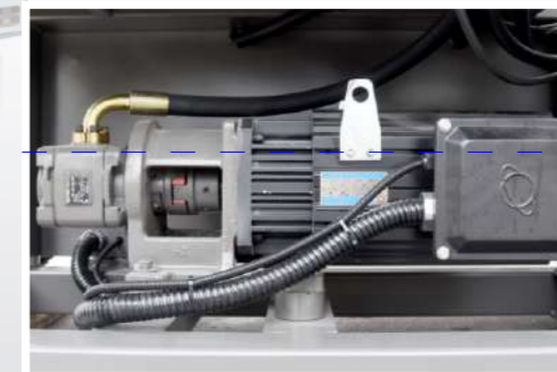
Servo motor and gear pump
