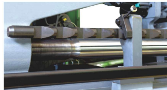
Auto-adjust mechanical safety bar
